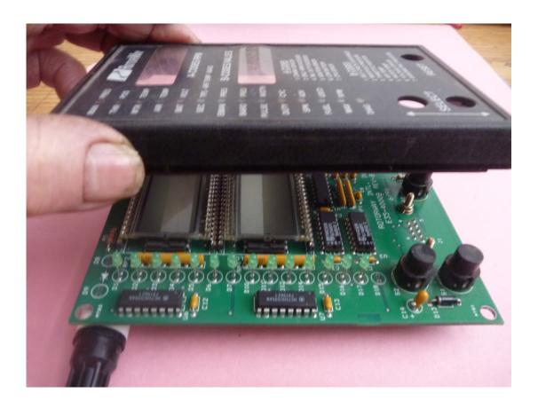
Now comes the tricky part. Gently lower the front cover onto the board. The trick is to get the 4 corner posts, the 3 push-buttons and all of the green LEDs to line up with their respective holes. Do not use any force. If you gently jiggle and rock the cover, and hold your tongue just right, it will fall into place.
